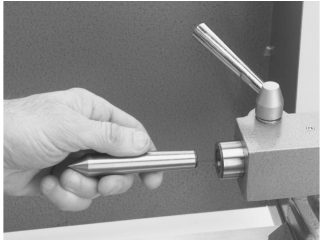
Inserting dead center into tailstock barrel
