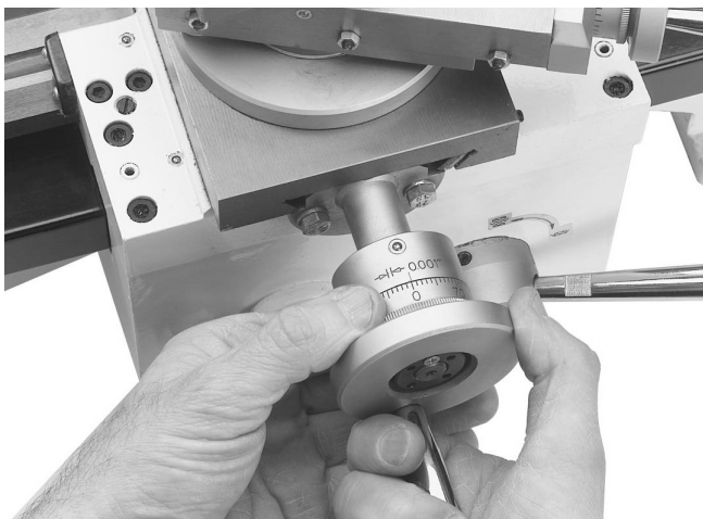
Adjusting handwheel scale
