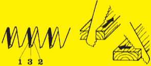
For cutting across as well as along fibres. With three edges that give faster sawing and a cleaner cut.
