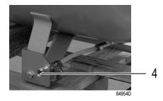
Condensate drain valve on air receiver
