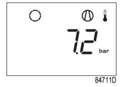
Main screen with shutdown indication, element outlet temperature
