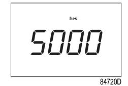
In the example shown, the screen shows the unit used <hrs> and the value <5000>: the controller module has been in service during 5000 hours.
