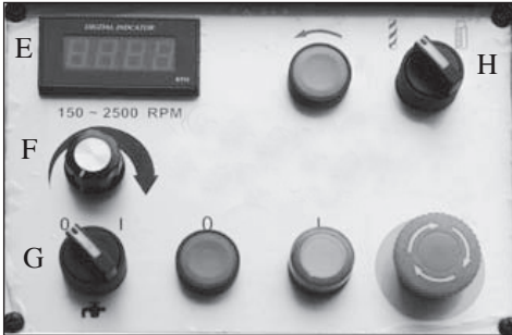
Fig. 1 !Warning: After daily use, disconnect machine from power source or press emergency stop switch to shut off the power completely. Do not keep the machine connected over 24 hours, it may cause damage to the machine
