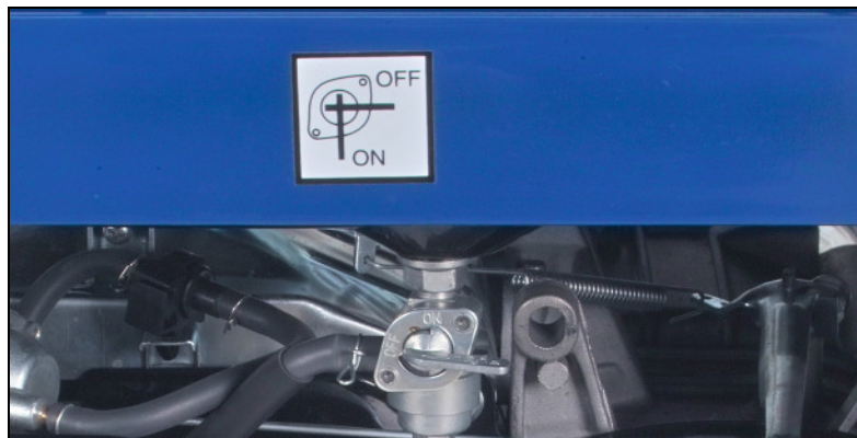
Fig. 4.6: Shut the fuel valve
