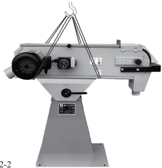
Fig. 2-2 Transportation sketch with a crane (After unpacking)
