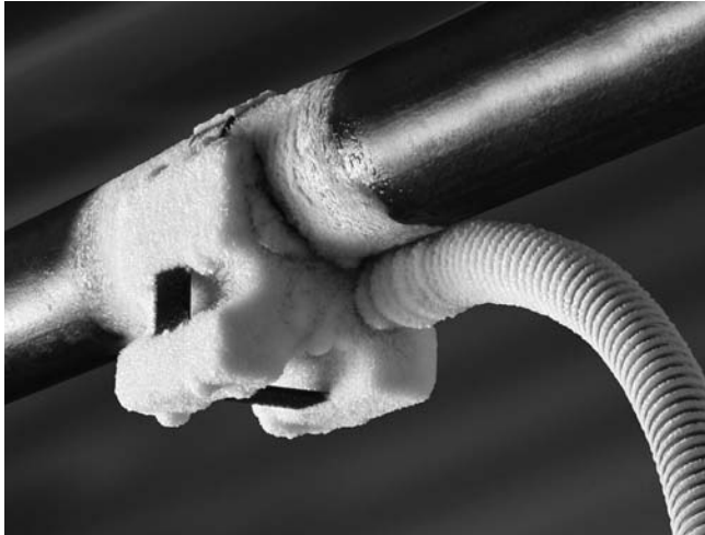
Figure 9 – Freeze Head Frozen to Pipe
