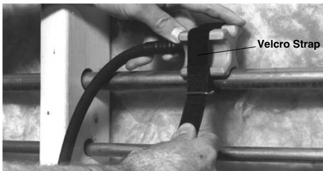
Figure 5 – Applying Freeze Head with Velcro Strap
