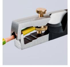
Induction-hardened shear blade with precisely ground cutting edges for crush-free cutting of copper and aluminium Lock nut prevents any unintentional adjustment cables of up to Ø 15 mm (5 x 2.5 mm²)
