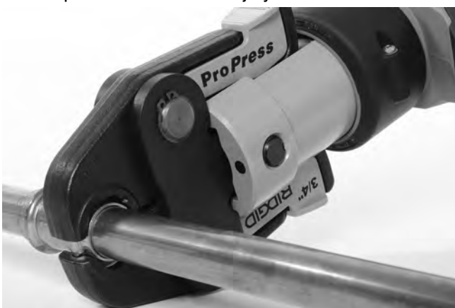
Figure 9 – Placing Scissor-Style Jaws Around Fitting
