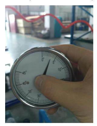
4. Set installed the protractor, fasten the screw, and make the blade to  $45^\circ$ . Check to make sure the pointer between  $45\text{-}45.5^\circ$  .Then It will be okay.
