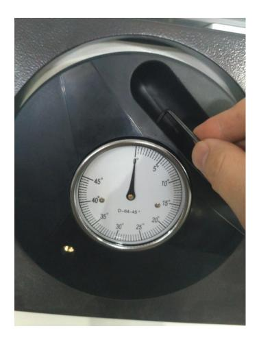
3. Take the protractor Vertical, make the pointer to 0  $\,^\circ$
